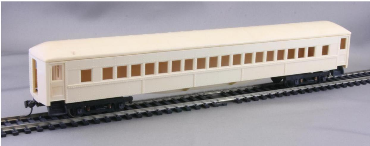
Figure 7. Finally, the roof and carbody were assembled using a jewelers' screwdriver through that hole in the center of the floor (Figure 4) to access the screw in the brass channel (Figure 5). And yes, those are Central Valley trucks. A few years ago, when
